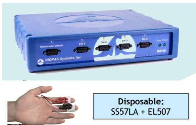
Fig. 2. Biopac data acquisition system (top) and leads with electrodes (bottom; https://www.biopac.com/wp-content/uploads/EDA-Guide.pdf )
