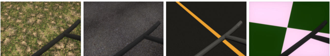
Figure 1. Sample images from Experiment 1 modelled in Autodesk MAYA 2016. Four terrains were created: grass, stones, runway and cross. In each image, the same helicopter skid was visible and used as a relative reference point. The images shown here depict an altitude of 5ft from skid to ground.
