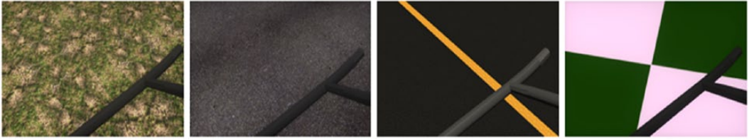
Figure 1. Examples of the terrains used in the low hover altitude estimation task. Each image was rendered in Autodesk MAYA™ 2016 at a simulated altitude of 5 ft or 1.5 m (from skid to ground). The terrains from left to right are the grass, stones, runway, and grid terrains, respectively. The same helicopter skid was visible in each image.
