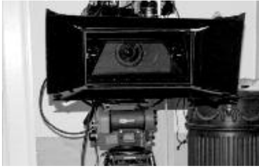
FIG. 1 A frontal view of a mirror rig shows the lens of the camera which films through the partial (beam splitter) mirror, as well as the reflection of the lens of the second camera that would record the image reflected off it. The distance between the two lenses is the inter-axial distance (IA). If there was no horizontal separation and lenses were vertically aligned as well, only one lens would be seen.
